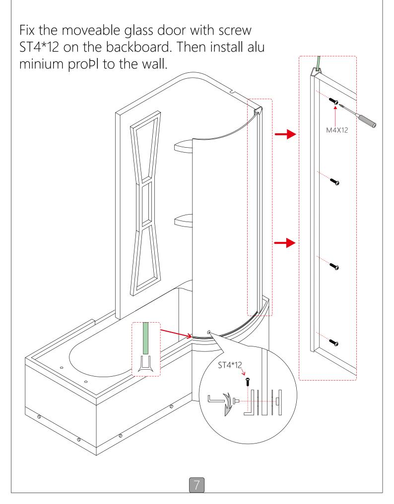
Fix the moveable glass door with screw ST4\*12 on the backboard. Then install alu minium probl to the wall.
