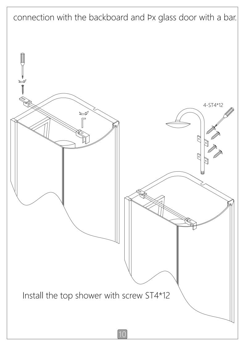
Fix the moveable glass door with screw ST4\*12 on the backboard. Then install alu minium probl to the wall.
