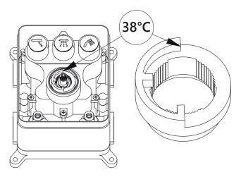
3. Place the temperature control ring back in the 12 o'clock position.
