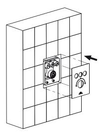
8. Before fitting the handle please read instruction of the TEMPERATURE SETTING and if everything is suitable then install the handle completely.
