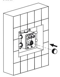
5. With shut-off valves installed inside the faucet on the sides (1-HOT and 2-COLD) you can adjust or close the flow of hot and cold water to the faucet with the help of a screwdriver.
