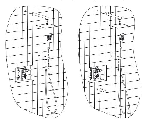
4. Open the water supply to check that each connection is tight, there are no leakage and free of cracks.
