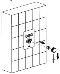
2. There are 2 marked lines on the thermostatic cartridge, keep them in one line. If we turn the axis of the thermostatic cartridge clockwise – the water will flow cold, if we turn it counterclockwise – it will be hot. The more we turn counter-clockwise or clockwise, the colder or hotter the water will flow, respectively.
