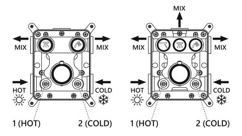
6. By turning the thermostatic handle to the end position clockwise, this is the maximum cold water (C) temperature position, make sure that the water flows cold. By turning the thermostatic handle to the end position counter-clockwise, this is the maximum hot water (H) temperature position, make sure that the water flows hot (use a thermometer).
