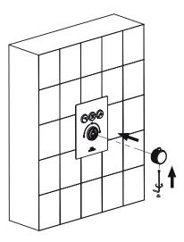
9. To start the water press the corresponding button (see figure with button markings). To start cold water, turn the thermostatic handle clockwise, for hot water – turn the handle counterclockwise by pressing the knob on the handle.
