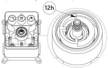
4. Place the handle so that the knob button is at 12 o'clock position and secure it with the screw. Insert a decorative plate into the hole in the handle.
