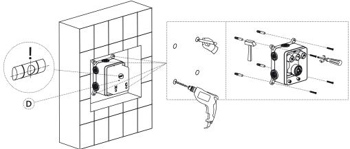
2. The hot water supply inlet (on the left side of the faucet (box) (HOT)) must be connected to the hot water supply system and the cold water supply system (on the right side of the faucet (box) (COLD)) must be connected to the cold water supply system. Connect all outlets to the markings on the large upper shower head / small shower head / spout buttons.
