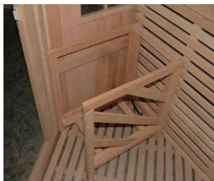
FIG-16 disassemble the wooden frame
